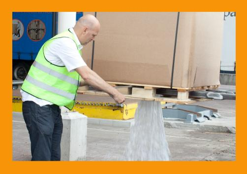
The speed of the discharge depends on the viscosity of the product. The unit will empty completely and very little product is left in the unit. If desired the last bit can always be squeezed out later, when the bag has been removed from the unit.
