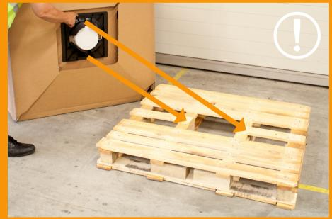
Place the unit with cassette on the pallet and make sure the open spaces in the positioning plate fall directly in the top shelves in the center of the pallet. The unit will then always be positioned correctly on the pallet.
