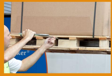
With the first shipment of the Conicube, you will receive a long key, which operates the valve. This special key has four equal, special shaped sides. Align this key with the inside profile of the spindle of the valve. Insert the key in the spindle until it reaches the end of the hole.
