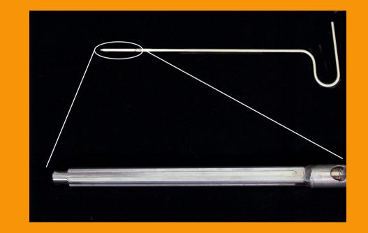
profile of the spindle of the valve. Insert the key in the spindle until it reaches the end of the hole.
