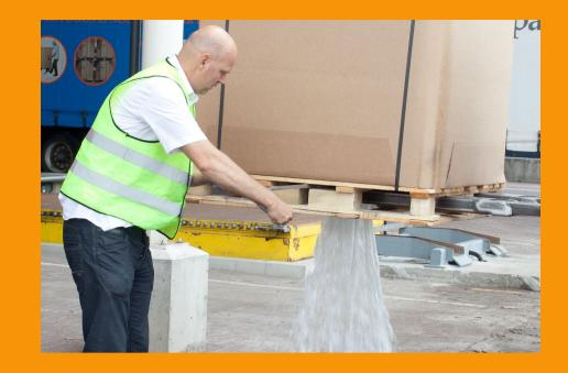
8. The speed of the discharge depends on the viscosity of the product. The unit will empty completely and very little product is left in the unit. If desired the last bit can always be squeezed out later, when the bag has been removed from the unit.
